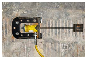
Typical shear test setup.
